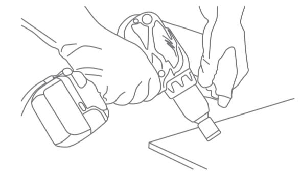
You can use cutting discs fitted to battery-operated screwdrivers or angle grinders, or electrical drills as an alternative.
