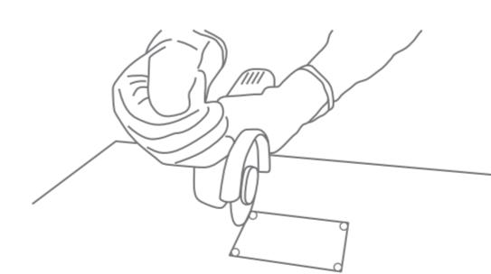
To get internal and L-shaped corners & to reduce the risk of breakage, cut 'o' at the vertex of the internal corners using bits with a radius of at least 5mm. Then cut with diamond discs, be cautious to stop moving the cutting tool forward. To drill and cut using diamond discs, and more follow the instructions provided below:
