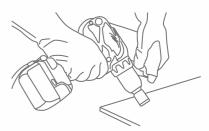
$You \ can use \ cutting \ discs fitted to battery-operated screwdrivers \ or angle \ grinders, electrical \ drills \ as \ an \ alternative.$
